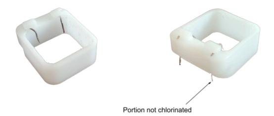
2. Take the two plastic PMMA parts, clean them with 100% Isopropanol and dry (top figure). Place them on a flat and clean surface (e.g. inside a petri dish). Position the two cleaned gaskets on the plastic piece aligning them in the half cavity (one gasket in each flowcell side, bottom figure). Important note: to prevent leakage in the flow cell final assembly, make sure the gaskets are perfectly dried before installing.
