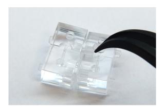
**3.** Center the chip on top of one of the gaskets as shown below. Ensure proper alignment of the chip (3 mm). Important note, if you treat the chip with a wetting solution such as Piranha, ensure thorough drying before installing it into the flow cell. Failure to dry the chip adequately may result in leakage issues during the final assembly.
