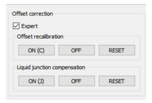
Pressing the **ON** button will activate the offset recalibration procedure on the selected channels (and will append the letter C to their labels in the **Channels Overview**). This procedure has to be performed in open circuit, i.e. with no load connected to the amplifier's input. The offset recalibration estimates the current offset and subtracts it, so that the current in open circuit is as close to 0 as possible.
