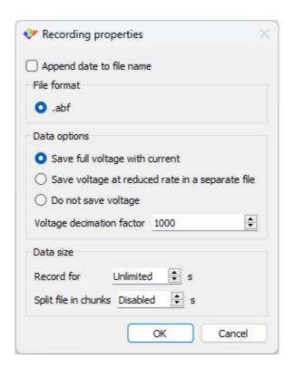
NOTE: Certain devices have a very high throughput. Since both currents and voltages are saved in the same file by default, the user can choose not to save the voltages (making the files 50% smaller), or to downsample the voltages (making them practically irrelevant in size but still usable for analysis).
