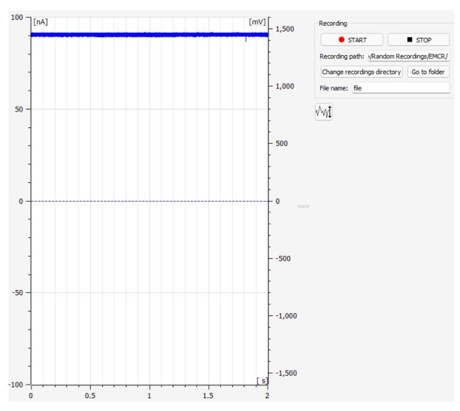
The central window of the Graphical User Interface displays the acquired input current channel (or channels for multichannel devices) and the control voltage in an oscilloscope-like fashion.
