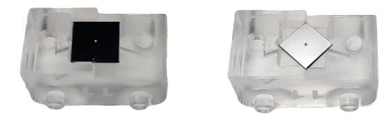
**4.** Next, place the second gasket on top of the nanopore chip. Even in this case, note that the alignment is different for 5x5 (left figure) and 4x4 chips (right figure).
