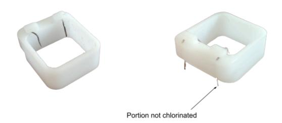
2. Choose one of the transparent plastic parts, clean it with 100% Isopropanol and dry. Place it on a flat and clean surface (e.g. inside a petri dish). Position one of the cleaned gaskets on the plastic piece as shown below. Important note: to prevent leakage in the flow cell final assembly, make sure the gaskets are perfectly dried before installing.
