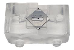
**5.** Sandwich the assembly between the two transparent plastic pieces, feeling the compression of the gaskets.
