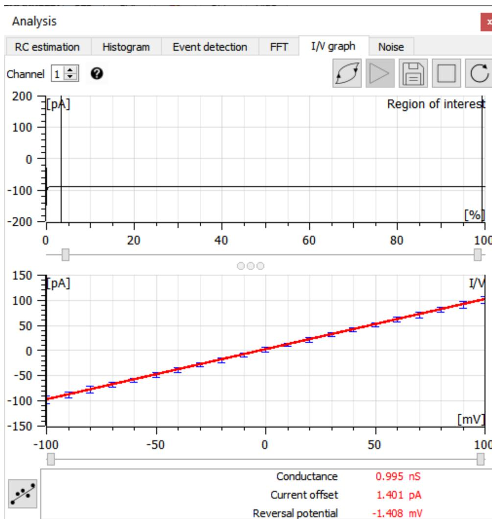
Clicking the linear fit button
