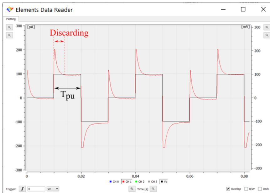
Capacitance is estimated considering the equation  $C = \Delta I / \Delta(dV/dt)$ , so considering the current jump corresponding to the voltage slope change when the triangular wave crosses a minimum or a maximum.
