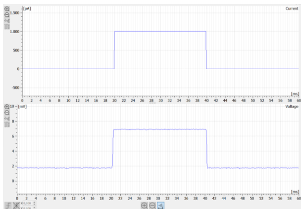
Before bridge balance
