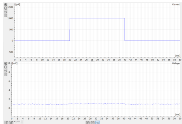
After bridge balance
