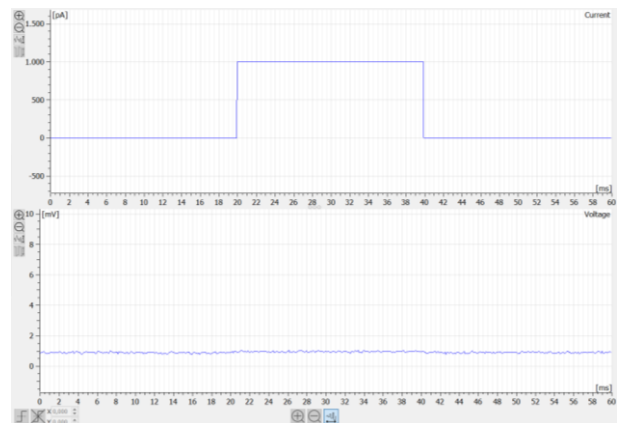
After bridge balance
