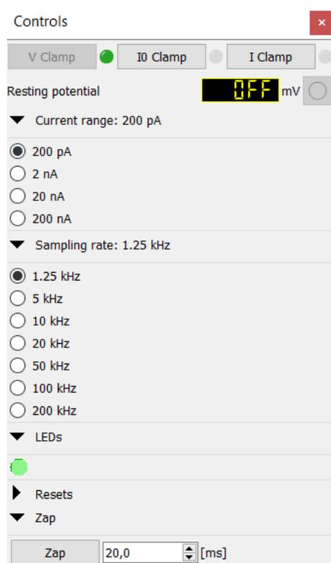
**Acquisition modes:** three operating modes are provided. Voltage clamp, true zero current mode (I0 clamp) and current clamp. The I0 Clamp mode clamps the pipette current to zero enabling the voltage recording with no current. When I0 mode is selected, the resting potential of the impaled cell appears and updates in real time within the display located below the commands; in addition, the recording button next to the display becomes available to save the recording to disk as a .abf file.
