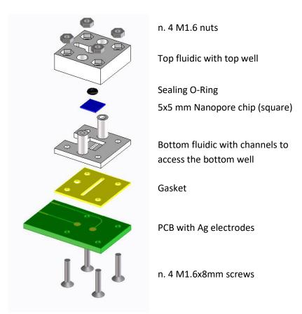
Two kind of nanopore chips are availbe, both with a SiN layer where the nanopore is drilled, but one type is glass-based and the second type is SiO based. The thickness is different between the two nanopore chip, and it's 200  $\mu$ m for the glass based and 500  $\mu$ m for the SiO, so please use the correct bottom fluidic part with the correct nanopore chip thickness.
