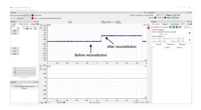
It may happen that the protein inserts just after the membrane painting. This causes an expected dramatic change in the current response waveform (see image below), as a resistive component (the alpha hemolysin) inserts into the RC circuit.
