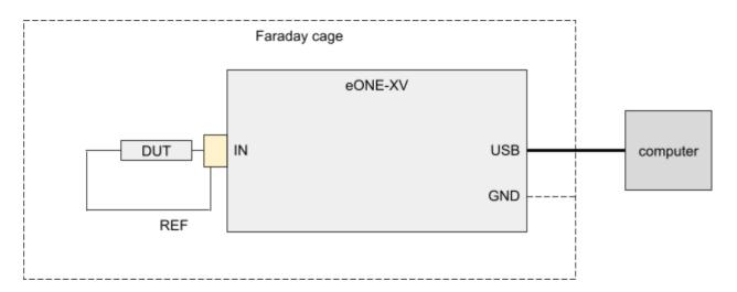
The scheme below shows how the control voltage is applied and the polarity of the acquired current.
