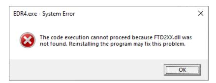
The FTDI driver actually ends its installation only when one device is plugged to the computer via the USB cable. Until then the driver cannot finish its installation and so the software cannot start.
