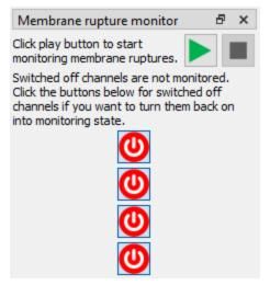
The control has a button for each current channel that can be clicked directly by the user (in which case it works the same exact way as switch off buttons near the current plots), or that is automatically triggered by the control when a persisting saturation is detected, once the start button is pressed.
