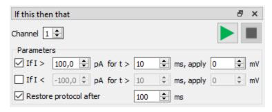
The Channel field can be used to select a specific current channel to monitor, or it can be set to channel in order to monitor all channels.
