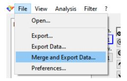
In the window that will appear select the source datasets by dragging them from the Available Data panel to the right panels. Doing this remember that you have to select exactly one dataset to inherit voltage data from. Then, as for the regular export select the path, the filename, the file format and click ok.
