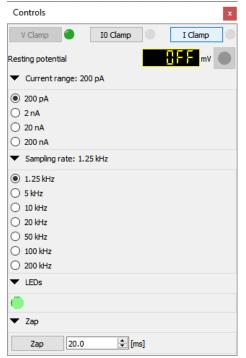
enabling the voltage recording with no current. When I0 mode is selected, the resting potential of the impaled cell appears and updates in real time within the display located below the commands; in addition, the recording button next to the display becomes available to save the recording to disk as a .abf file.
