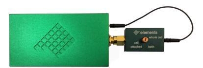
Rotate the selector of the model cell until the small arrow points to the "bath" configuration label.
