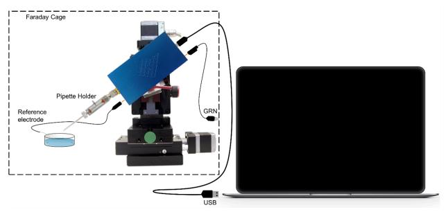
Mount the ePatch on the micromanipulator using either the dovetail or the rod bar mounting system.
