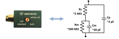
Use the drop-down menu of the "membrane test widget" to display the analysis of the membrane transient (whole-cell option). The real time analysis of the current response defines the values of the membrane capacitance (CMembrane), the membrane resistance (RMembrane) and the series resistance (RAccess).
